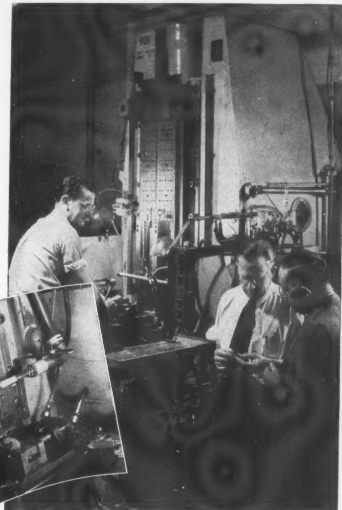
The Department Foreman consults with a Gulf Lubrication Engineer (right) on results with Gulf L.S. Cutting Base in broaching various business machine parts.
